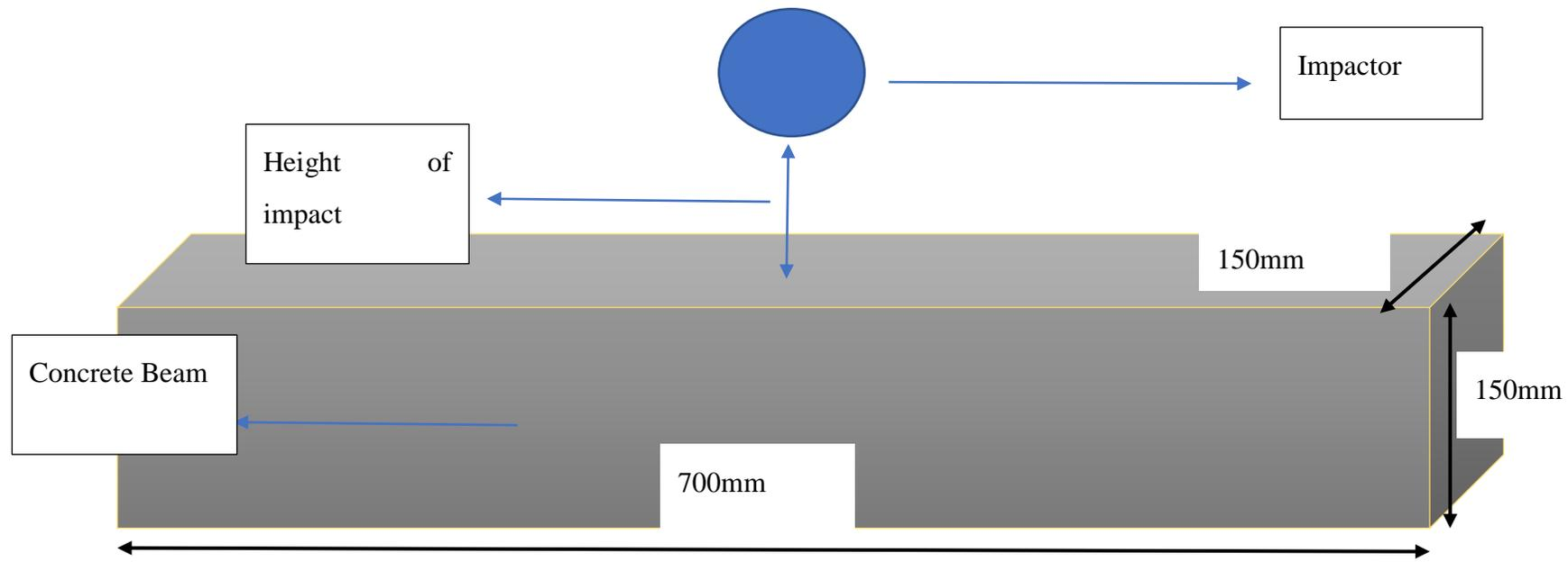
**Block Diagram of the test frame**
