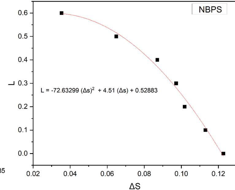
Variation of  $L$  vs  $\Delta S$  for different sensors configurations
