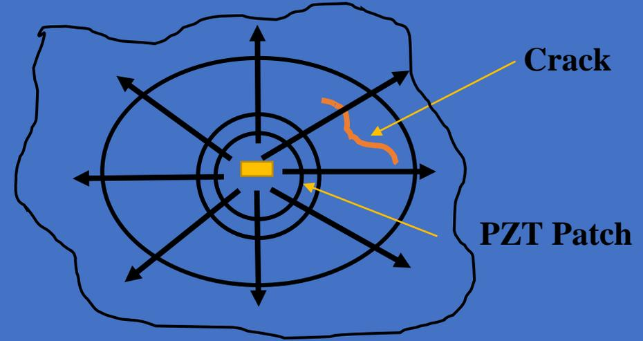
Cracks disrupts wave propagation
