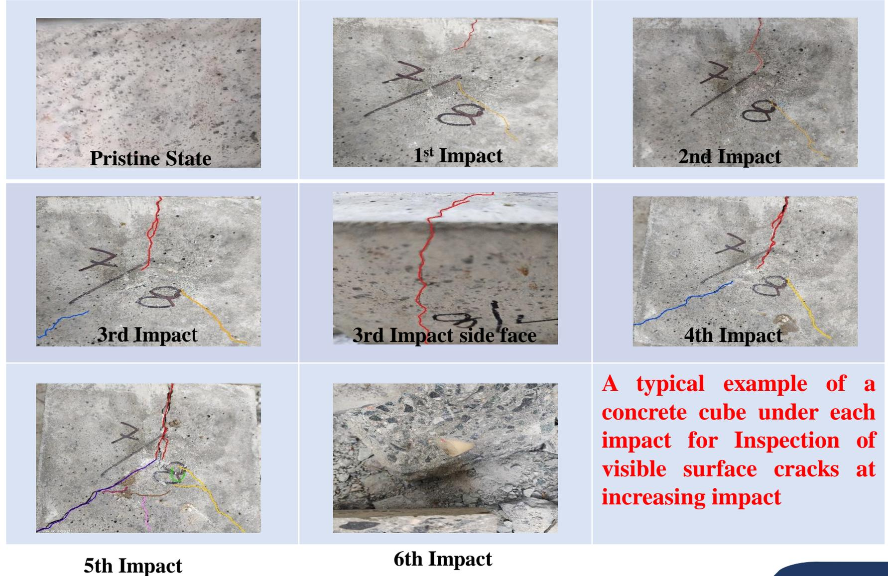
A typical example of a concrete cube under each impact for Inspection of visible surface cracks at increasing impact
