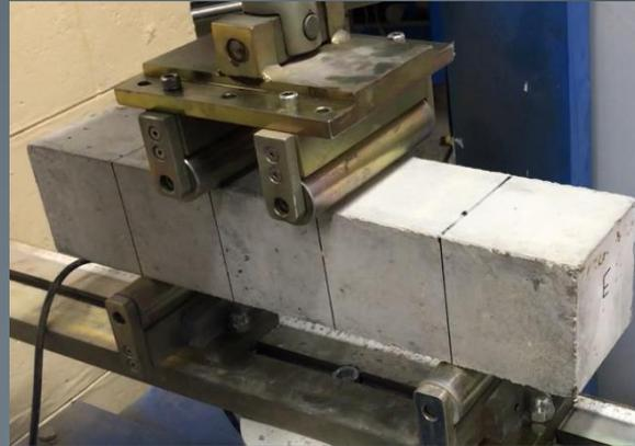
Modulus of rupture Test
