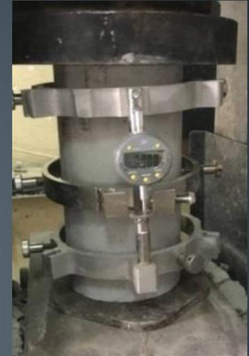
Modulus of Elasticity Test
