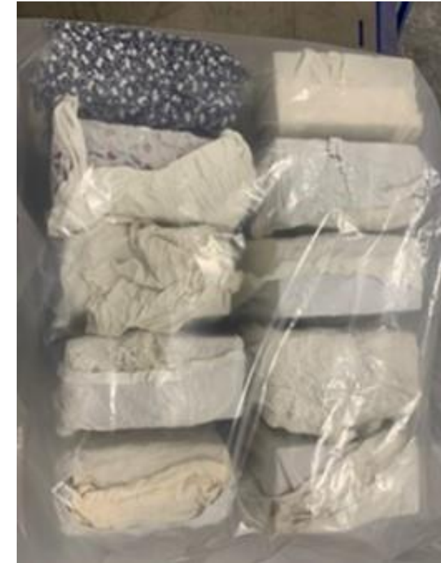
Specimens during for curing
